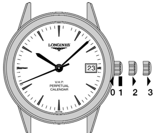
This watch is a product of advanced electronic and micro-mechanical technologies for everyday use. The L546 VHP movement is 20 times more precise than a conventional quartz movement, displaying the hours, minutes, seconds and date, and showing on demand the number of the month followed by the leap-year cycle in Roman numerals I to IV.
